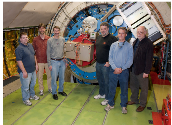
Fig. 6. Main cabin looking aft toward the pressure bulkhead and telescope assembly showing the facility class FORCAST imager mounted at the Nasmyth focus and members of the FORCAST Team. Left to right: Joe Adams (Project Scientist), Luke Keller (co-I), Terry Herter (PI), George Gull (Lead Engineer), Chuck Henderson (Mechanical Engineer), and Justin Schoenwald (Software Engineer). (NASA photo).
